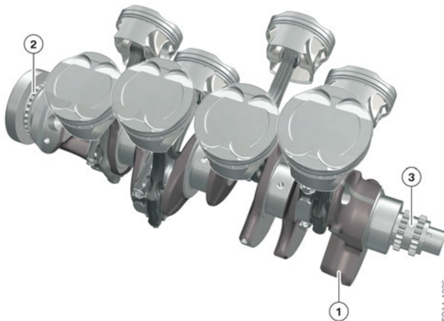
N63TU2 engine, crankshaft drive with connecting rod and piston
